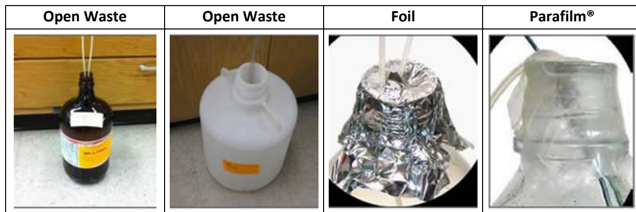
Figure 3.4 – Improper LC Waste Collection Practices
