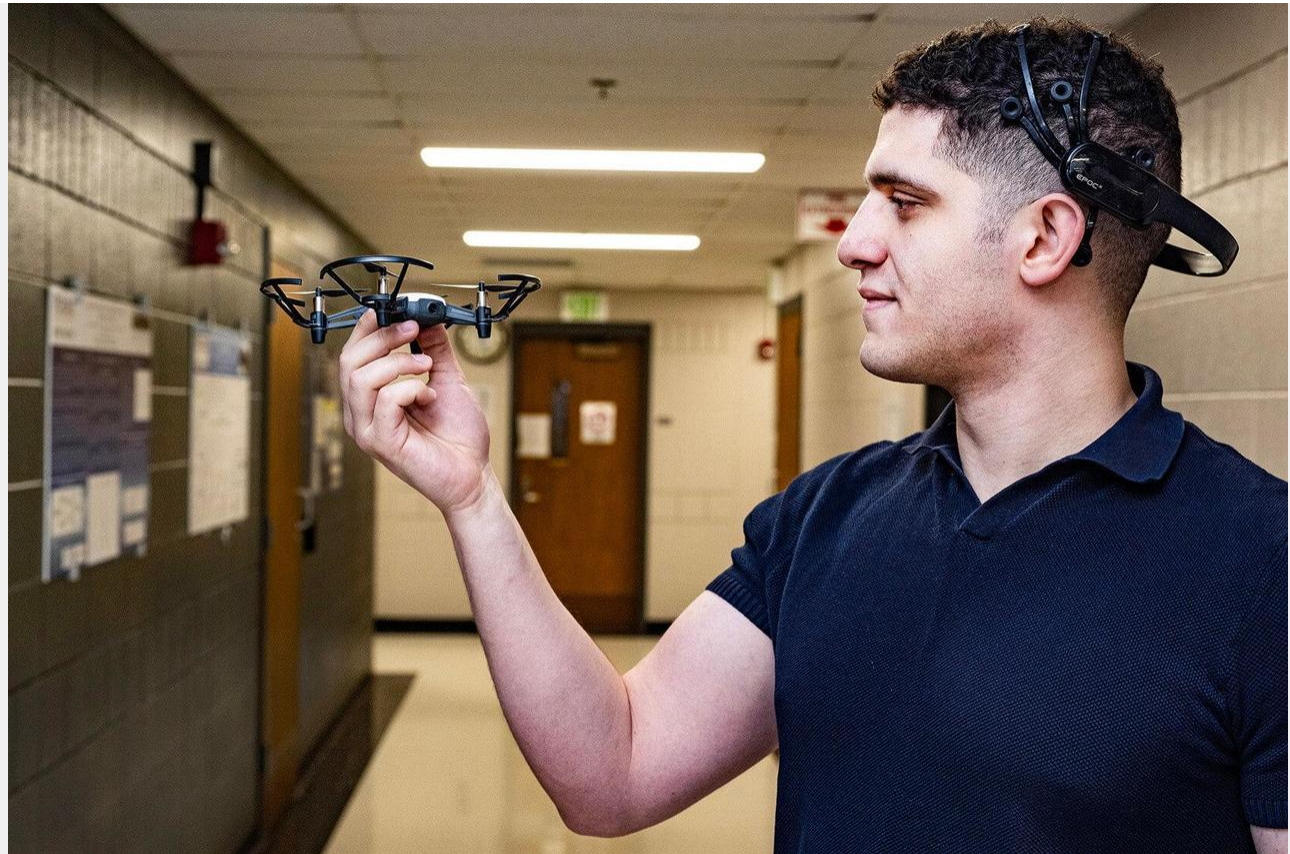
Graduate student Abdelrahman Gad inspects a small, four-propeller drone while wearing a headset that allows him to control it.
